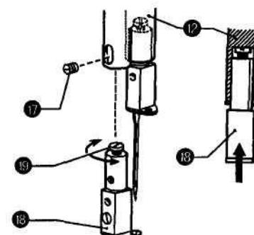
★ Insert the needle clamp all the way into the needle bar.
